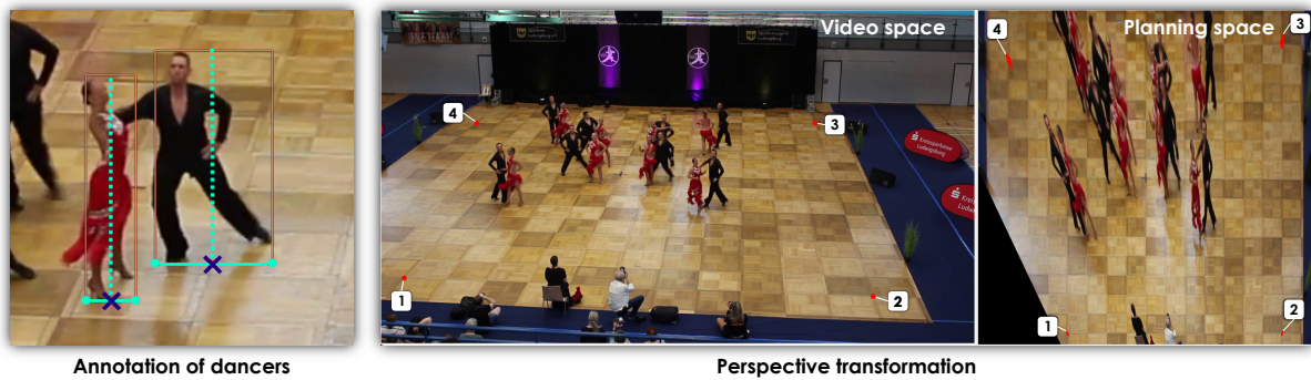
Figure 3: Bounding box annotation for individual dancers, the 2D position is determined by the center-bottom point of the bounding box. Coordinates are then transformed from video space to planning space for comparison with the planned formations.
