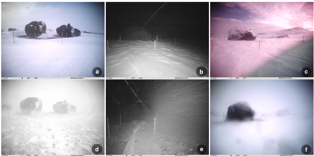
Figure 2: Example images from our input datasets, demonstrating the variability in the image quality, caused by different weather conditions. (a),(b) Good quality day and night images; (c) color distortions caused by sun; (d),(e) day and night images during snowstorm; (f) camera is partially covered by snow.
