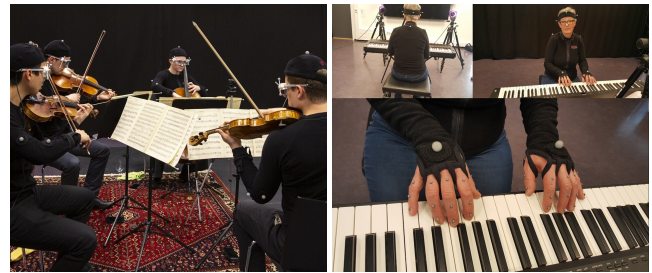
Figure 4: The left image shows musicians playing violin, motion captured using an optical MoCap system with reflective markers, tracking their body and instrument motion (image extracted from [Fut]). The right image shows a musician playing piano, while the movements of the finger joints are tracked with 5mm reflective markers (image extracted from [Ger]).
