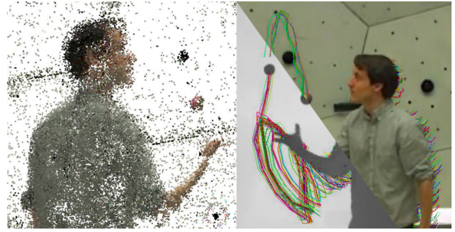
Figure 14: Dynamic View Synthesis by Tracking 3D Gaussians. (Left:) Gaussian centers; (right:) Rendered image and depth from unseen view with 3D trajectories (including occlusions). Luiten et al. [LKLR24] parameterizes each scene with 200 to 300k Gaussians, tracked across frames with an accuracy 10x better than previous state-of-the-art while also rendering at 850 FPS. Image source: [LKLR24] ©2024 IEEE.
