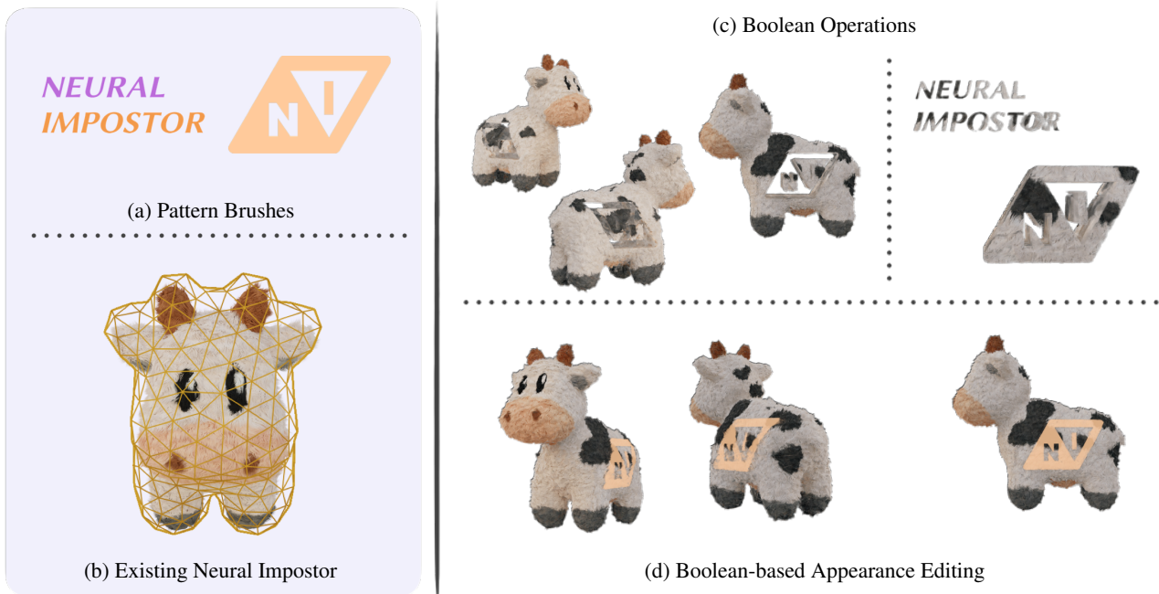
Figure 7: Boolean operations on Neural Impostor with given patterns. (b) Geometric difference and union based on the density of the given pattern. (c) Implicit union operation for color editing.
