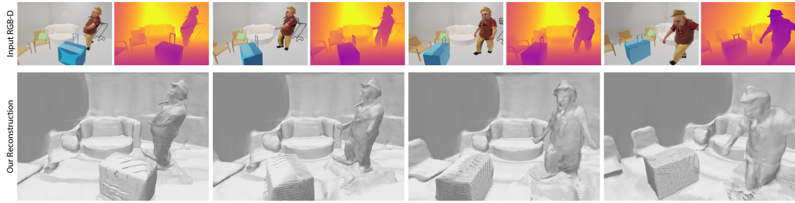
Figure 9: Dynamic scene reconstruction. We demonstrate our full scene reconstruction exhibiting non-rigid object deformation across different time indexes. Note how ours can recover plausible movement of the movement of the limbs across time.
