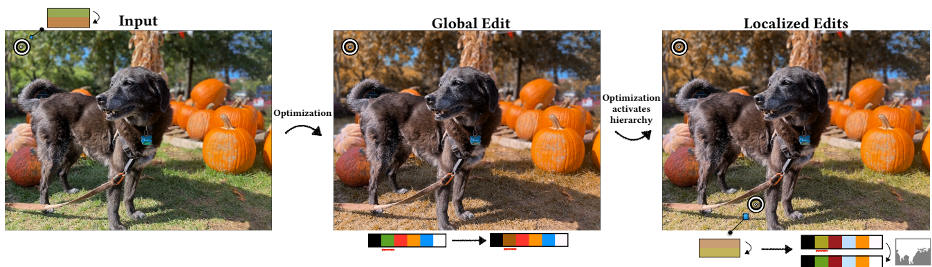
Figure 1: LoCoPalettes augments palette-based image editing with image-space constraints and semantic hierarchies. Left: The user places a spatial constraint on the input image to make the leaves brown. LoCoPalettes optimizes for a palette with respect to users' image-space constraints, shown as small white circles (Sec. 4.2). Center: The optimization updates the global palette. Right: The user places a second spatial constraint on the grass. If constraints cannot be satisfied with a single global palette, LoCoPalettes semantically segments the image and activates a palette hierarchy \mathcal{H} to achieve the color constraints using local palettes (Sec. 4.4). The grass constraint's semantic segmentation mask is shown in the lower-right.
