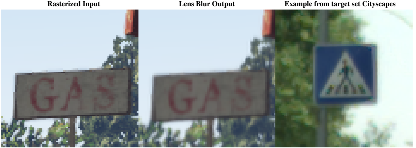
Figure 3: Example of the learned lens blur applied to a rasterized frame from the GTA5 dataset [RVRK16]. The jagged edges of geometry are mitigated by the learned kernel. The foliage in the background also looks more similar to the foliage in the target dataset.
