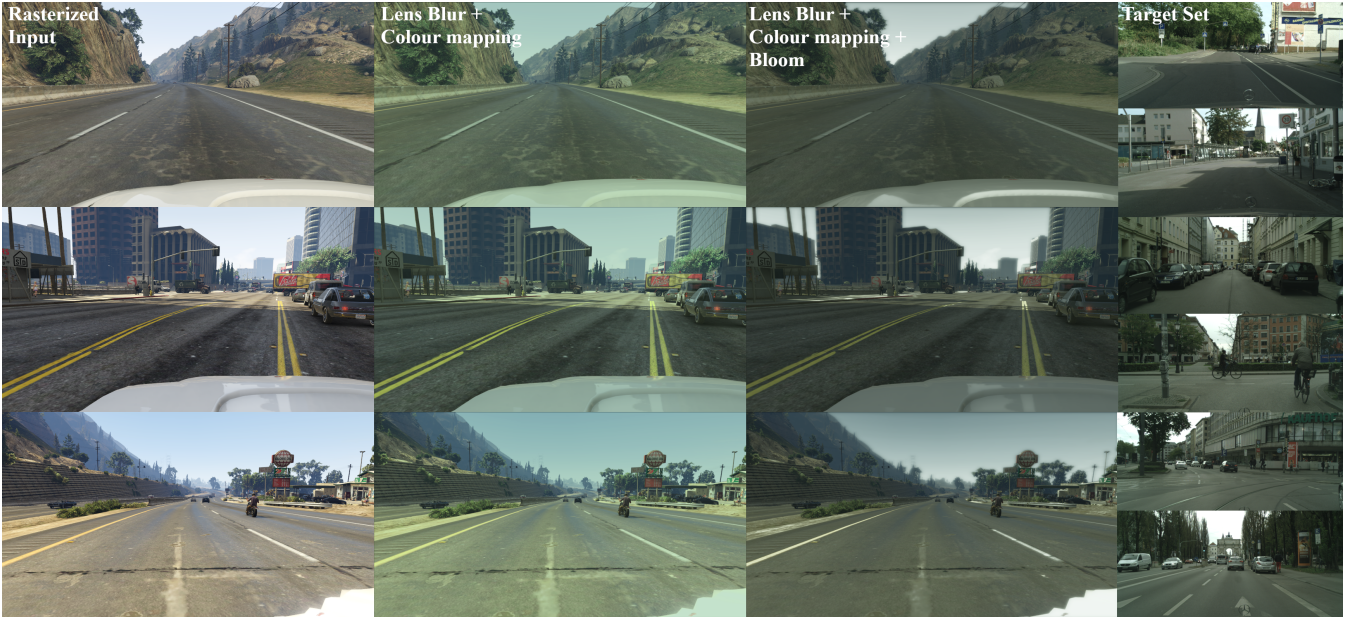
Figure 4: The color mapping function transfers the global color characteristics of the target dataset to the rasterized input frames. As well as replicating the "bleeding" effect caused by overexposure, by separately processing bright regions, the bloom shader helps prevent them from distorting the learned color mapping.
