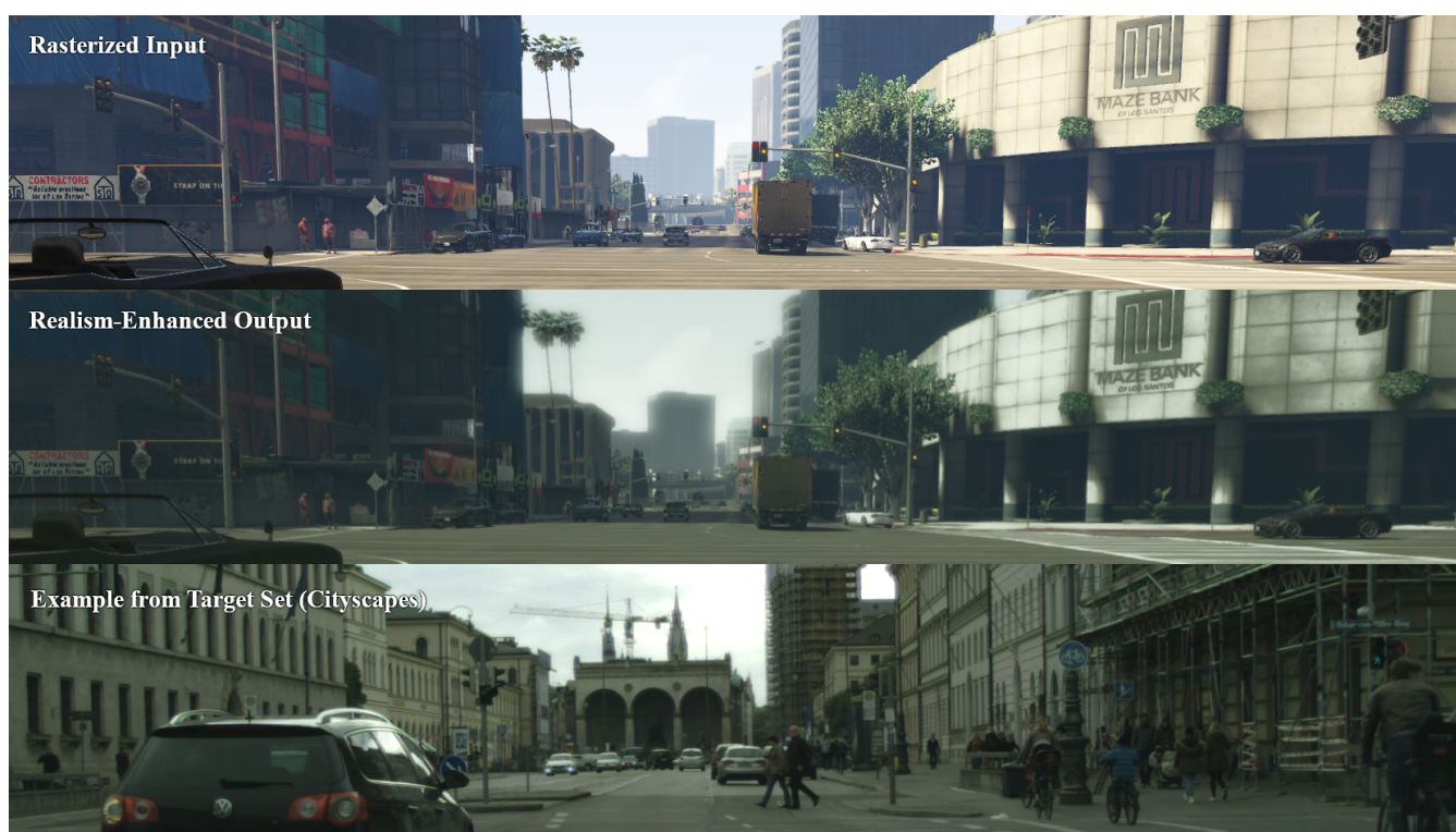
Figure 1: Our proposed Generative Adversarial Shaders combine the quality and automation of an adversarial training methodology with the computational efficiency and performance of a real-time post-processing shader pipeline. This crop is from a 1080p frame which was processed in 2.8ms on an Imagination Technologies BXT-32-1024 MC4 GPU to match the style of the Cityscapes dataset [COR* 16].
