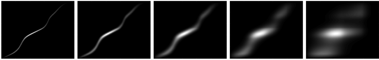
Figure 5: Solution to the problem of Fig. 1 with increasing amount of entropy. From left to right, the Gaussian standard deviation used in the convolutional approach of Solomon et al. [SdGP*15] is \sigma = 2, 5, 10, 20, 50 . As \sigma increases, the transport plan converges towards the trivial transport plan P(x, y) = f(x)g(y) .
