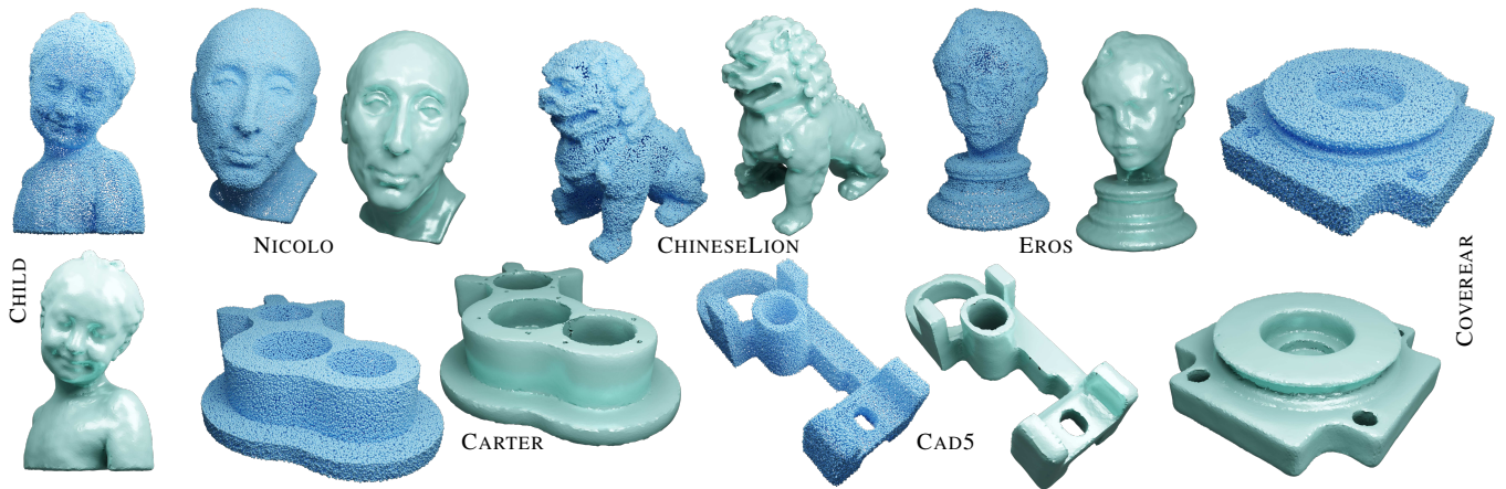
Figure 1: Denoising through line processes. By globally optimizing a robust and regularized fitting energy using line processes associated with local pairs of tangent planes, our method can robustly denoise raw point clouds (blue dots) while leaving features (if any are present) well preserved (green). Denoised pointsets are then visualized via their interpolating reconstruction through advancing front [DCS22] to offer a clearer visual evaluation of their (piecewise) smoothness.
