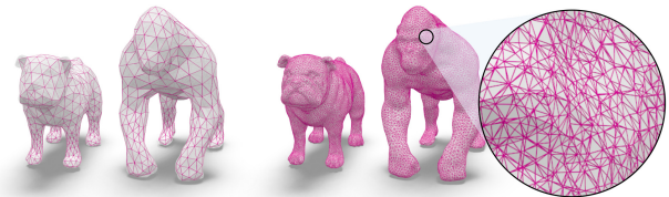
Figure 3: Approximating common triangulation with 581 vertices vs. overlay mesh with 105 677 vertices as map representation.
