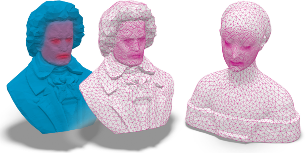
Figure 8: (left) Mesh \mathcal{A} with user-designed sizing field as input. (center, right) Common triangulation \mathcal{T} embedded on \mathcal{A} and \mathcal{B} , respecting the specified sizing.
