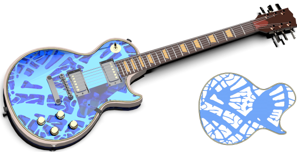
Figure 7: Optimized electric guitar body under planar-distributed loads, featuring spiderweb-like features.
