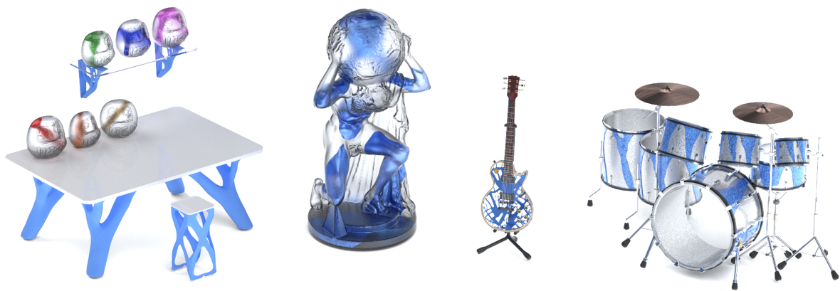
Figure 1: Structures with maximized stiffness and limited material consumption are optimized with low computation cost, all shown in color. The proposed NSTO also enables generating interpolated solutions with an instant network feedforward, like the seven drum shells.
