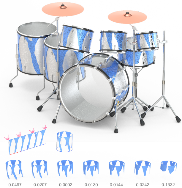
Figure 11: Solution space of drum shells, where diameter height ratio is the varying boundary condition. The top image shows the mapping between annular and planar structures, and the bottom image shows the solutions with latent codes.
