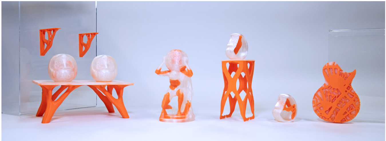
Figure 12: 3D-printed topology-optimized structures using the fused deposition modeling 3D printer (Ultimaker 3).
