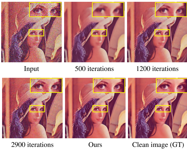
Figure 2: Denoising results produced by DIP [UVL18] with different numbers of training iterations.
