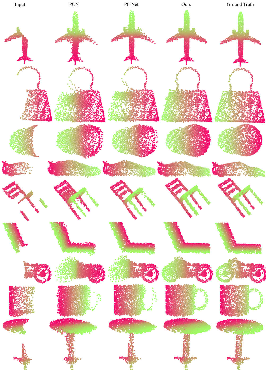
Figure 8: Visual comparisons. We compare our method with PCN, PF-Net, in 9 categories, including Airplane, Bag, Cap, Car, Chair, Laptop, Motorbike, Mug and Table. Our method has the best visual performance on average, which corresponds to the quantitative results.
