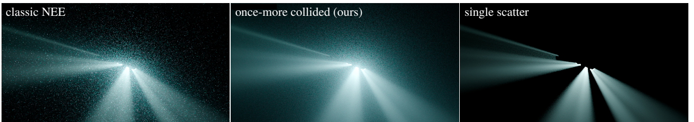
Figure 16: Once-more scattered next event estimation evaluated towards a light source, i.e. in path tracing from the camera. The images show the importance of the extra scattering vertex on top of single scattering only (right), and also demonstrate how our technique can robustly reduce the noise in this setting. All images are 1024 samples per pixel.
