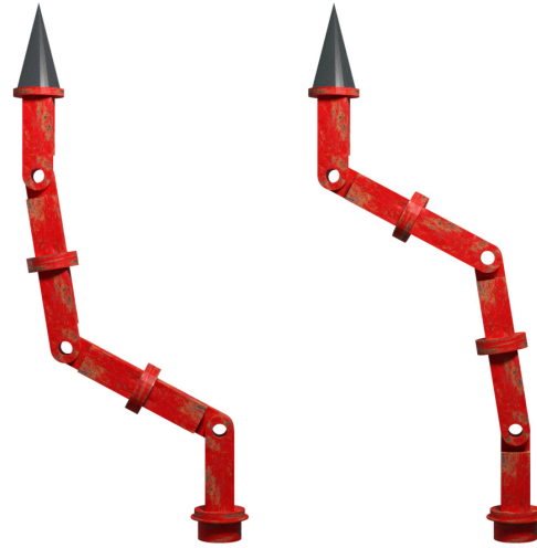
Figure 12: Robotic arm with two solutions: We show the robotic arm from Figure 10 and made an edit with some joints fixed to force the system to only be able to find two solutions. In this case the edit is not under-determined but there are two distinct solutions to the inverse problem and our system is able to find them during the global optimization phase. The solution on the left-hand side is the nearest solution i.e., the solution that changes the least the angles. The solution on the right-hand side is the farthest solution i.e., the solution with the biggest changes in angles. Note that the change that makes the right-hand side solution farther from the initial configuration is very subtle: the first joint (on the bottom) is rotated by 180 degrees.
