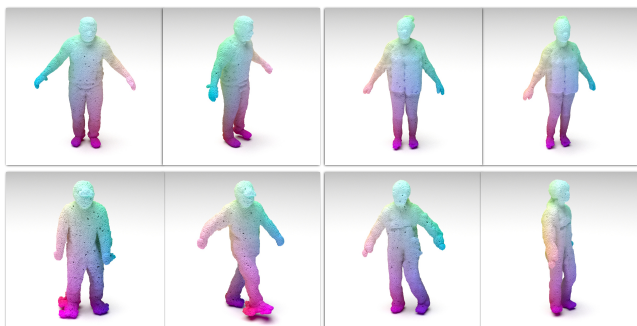
Figure 9: Each pair visualizes the dense correspondences derived from the backward motion flow between the canonical body (left) and the body reconstructed (right) at an observation frame.
