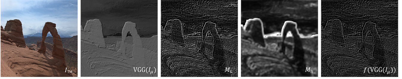
Figure 6: Feature contrast masking visualization of VGG feature maps (1st layer, 18th channel). From left to right: tone mapped image I_{TM} , original VGG feature map VGG(I_\mu) , feature contrast self-masking M_s , neighborhood masking M_n , and final f(VGG(I_\mu)) masking terms.
