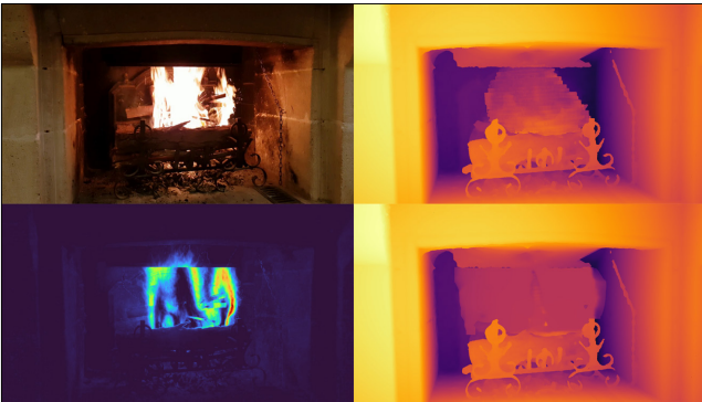
Figure 10: Total variation based depth propagation. For an input video (top left) we extract a median depth along the volumetric representation (top right). However, to assign plausible depth to dynamic video-specific regions not in the volumes, we propagate this depth (bottom right) using the per-pixel total variation as a guide (bottom left).
