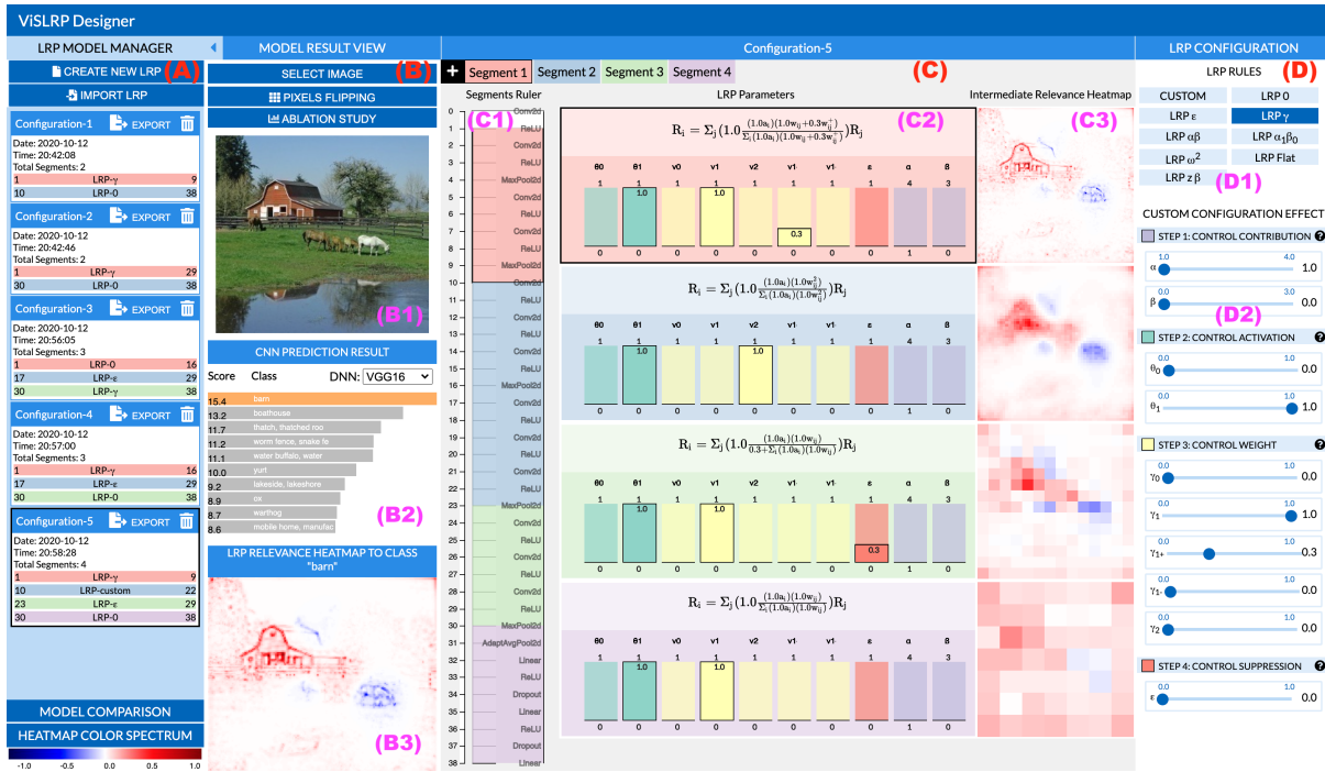
Figure 2: VisLRPDesigner interface. (A): Model manager for users to create, edit, and compare multiple LRP models, and to change heatmap color spectrum. (B): Model result view for selecting an image of interest (B1), checking CNN prediction results (B2), and studying LRP computed relevance heatmap (B3). (C): LRP configuration view which includes a segment ruler (C1) for users to drag and define segments, and LRP parameter view (C2) visualizing parameters of four segments, and intermediate relevance heatmaps (C3) after each segment. (D): LRP configuration panel for users to select a predefined LRP rule (D1) and customize LRP parameters in four steps (D2). Please note that VGG16 is used in the examples throughout the paper unless otherwise specified.
