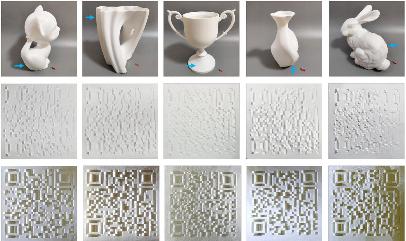
**Figure 25:** 3D-QR-codes printed on models with different geometries and light angles. Top-to-bottom are the 3D printed model and zoom-ins on the 3D-QR-code under the ambient and directional light environments. Models left-to-right: Kitten, Vase#1, Trophy, Vase#2, Bunny.
