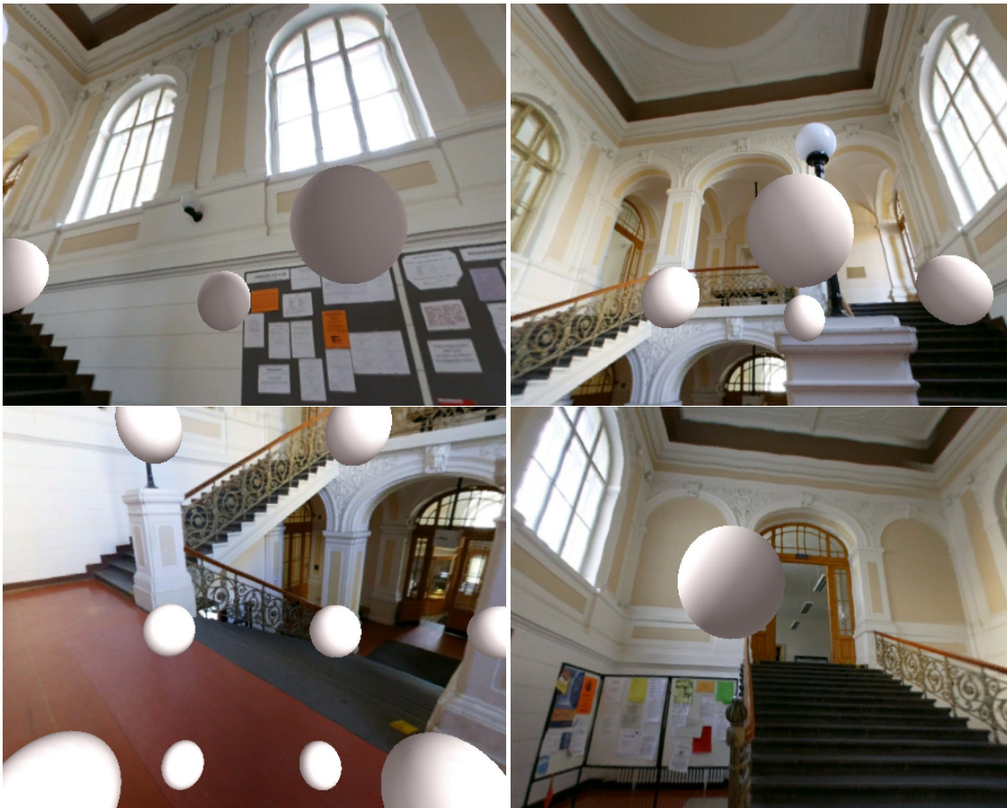
Figure 8: Four different views of the hall scenario with randomly placed white balls to illustrate the shading resulting from the estimated lighting conditions with ambient plus 4 directional sources. The views are rendered with a large field-of-view to make it easier to orient the views relative to the scenario, therefore the balls are sometimes distorted.
