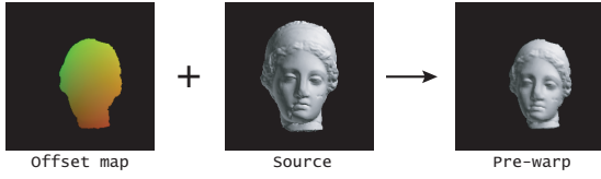
Figure 6: Pre-warp image generation from source image using offset map.
