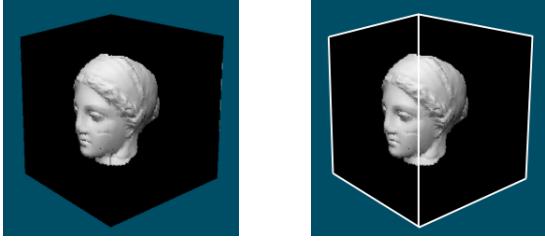
Figure 3: Object represented by relief texture mapping
