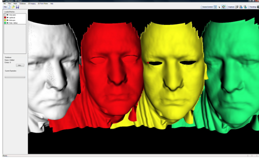
Figure 6: Comparative analysis of noise removal around the eyes from left to right: original mesh; fitting an elliptical mask around the eyes and filling with a spherical surface centered at 40mm behind the model; punching an elliptical hole around the eyes; filling the elliptical hole with bilinear interpolation
