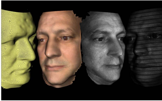
Figure 7: Triangulated mesh (left), with color and black and white texture mapping (centre) and with original stripe pattern (right)
