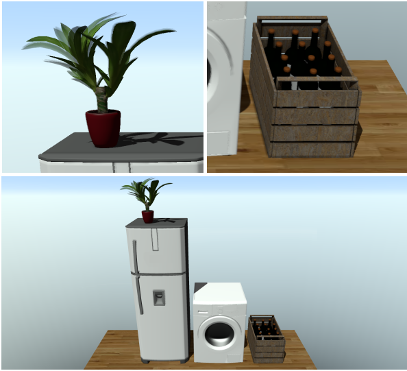
Figure 8: In this simulation, a washing machine is running, making the floor vibrate. Our contact responses make the bottles shake. The vibrations are also propagated to the indoor plant through the fridge.
