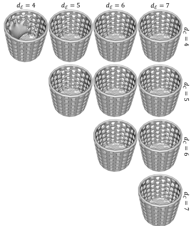
Figure 7: Comparison of the reconstructions obtained using a Dirichlet envelope with increasing rasterization depth, d_E , and increasing regular-grid depth, d_C .
