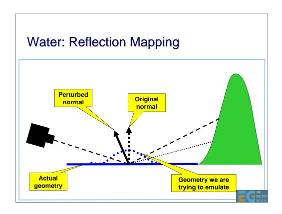
The viewer (camera) is on the left. The water is drawn as a flat surface (i.e. there is no geometry representing the ripples). To emulate the ripples, the normal is perturbed and this is used to modify the reflection vector.
