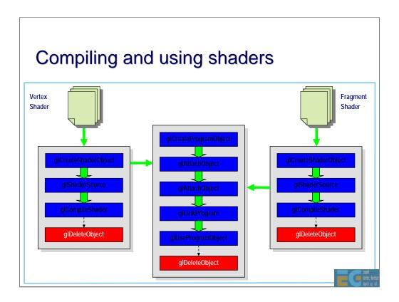
This shows the flowchart for compiling and linking shaders. GL is based on objects and each object must be explicitly created and deleted.
