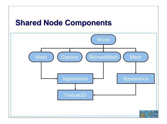
Even though nodes can't be instanced, their component objects can. Textures, vertices, and all other substantial data is in the components, and only referenced by the nodes.
