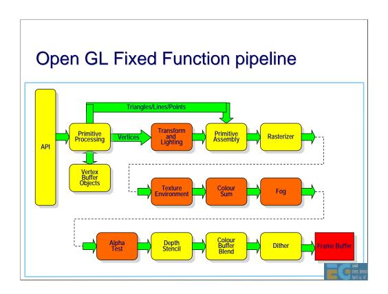
This shows the existing ES 1.1 pipeline. The boxes coloured orange represent the functions that will be replaced by shaders in ES 2.0. The transform and lighting block is replaced by the vertex shader. The texture environment, colour sum, fog and alpha test are all replaced by the fragment shader.
