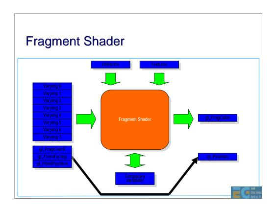
The fragment shader inputs the user-defined varyings, the fixed function variables and the fragment uniforms. The shader can read textures. It also has a set of temporary variables available. Like the vertex shader, these temporary variables cannot be shared.
