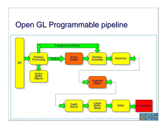
This shows how the vertex and fragment shaders fit into the ES 2.0 pipeline.
