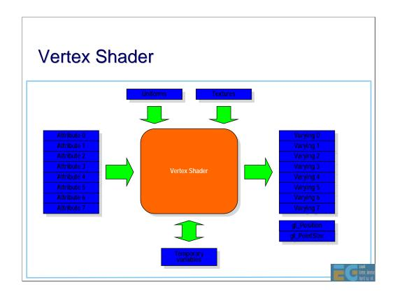
This shows the programmers view of the vertex shader. The (up to) 8 attributes are input on the left. Uniforms can be read by the shader. In some implementations, the vertex shader may also access textures. While the shader is running, it has access to a number of temporary variables. Note that these variables cannot be shared between vertices.
