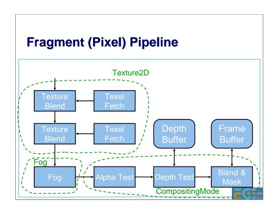
Here is a high-level view of the M3G/OpenGL fragment pipeline, and how some of the Appearance components map onto that. The other components would map to the transformation & lighting pipeline in a similar way.
