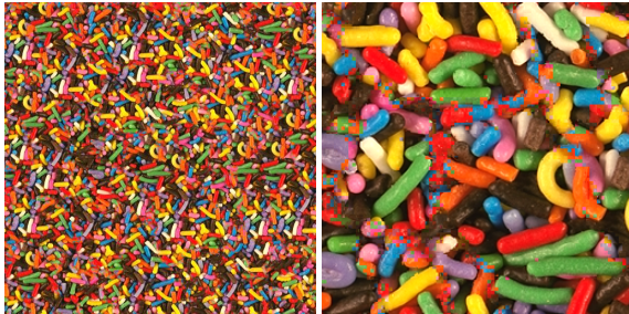
Figure 5: Colour assignment error at texture patch borders. Left: full synthesis result gives a good overall impression, right: a detail view of the texture shows the colour artefacts.
