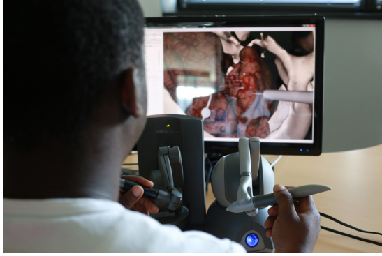
Figure 3: Photography of the set-up where a trainee uses two haptic arms to interact on the surgical physical simulation.
