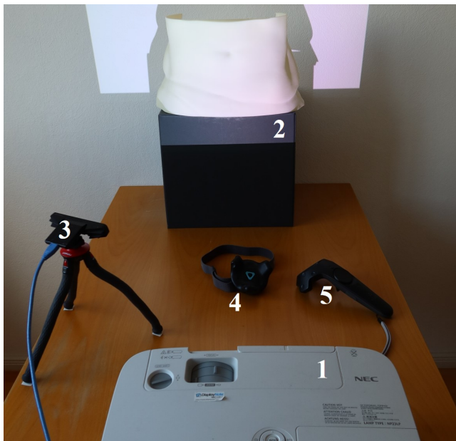
Figure 2: Setup for our projection system: standard projector (1), 3D print of abdominal skin (2), and RGB-D camera for object tracking and camera-to-projector calibration (3). The Vive tracker (4) and controller (5) will only be used for the extensions depicted in Sections 4 and 5, respectively. The camera position shown here is used for capturing most images of projection results throughout this paper.
