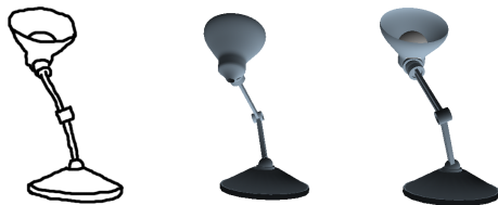
Figure 2: An example of the forward-backward ambiguity issue in inferred 3D pose of a lamp when not using the internal lines for additional information.
