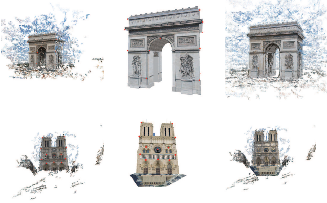
Figure 2: Registration process between the point cloud model and 3D surface mesh model. The first and second column represents the point cloud model and the 3D surface mesh model, respectively. In the third column, we render both of them after registration. For these two examples, the transformed 3D surface mesh model coincides with the point cloud model, which means that the registration algorithm is effective.
