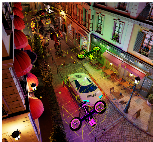
Figure 3: Each yellow box is the root node of a bottom-level acceleration structure (BLAS), here shown for the Bistro scene. Notice that both static light sources, e.g., the street lights and hanging light bulbs, and dynamic emissive objects are each represented by one or more BLASes, here in total 142 for the full scene.
