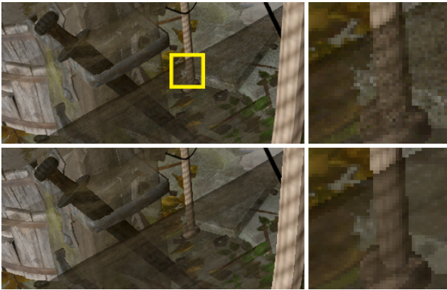
Figure 4: The blacksmith model comparing (top) MLCB with 32 coverage samples with (bottom) MLAB. In both cases, we use k = 4 .
