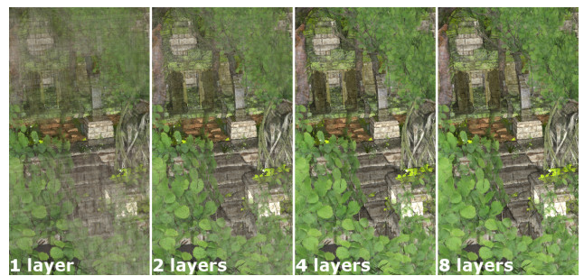
Figure 8: The Unreal Foliage Map, all surfaces \alpha = 0.75 , rendered with SLAB using b = 32 and varying numbers of layers.
