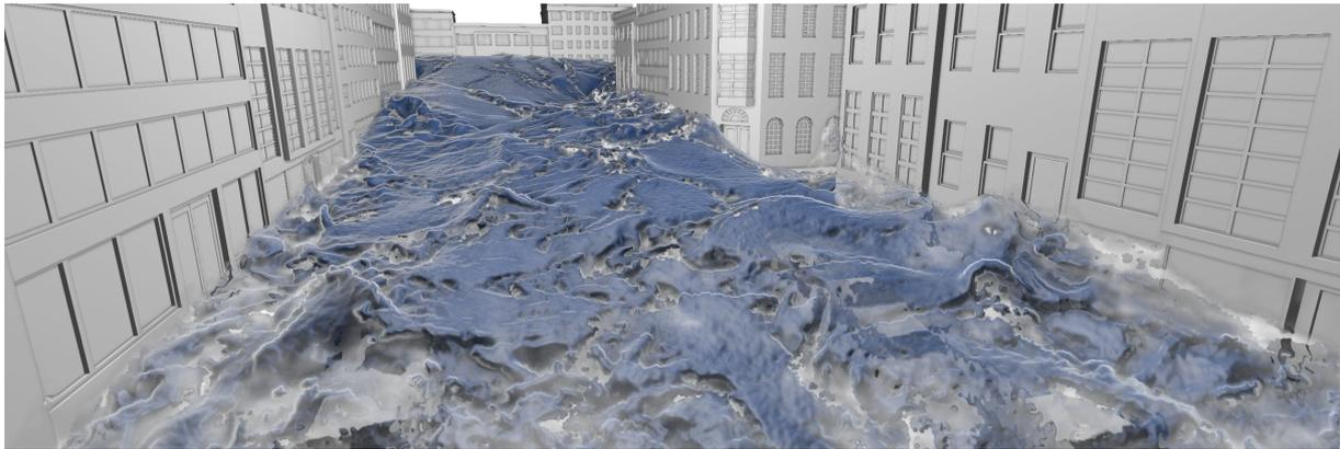
Figure 1: Rendering a 500 million particle simulation, preprocessed in 12 seconds, at 72 ms per frame on a  $1280 \times 720$  viewport using ray-sphere intersections, image-based surface smoothing, volumetric foam and approximative refractions on a single PC.
