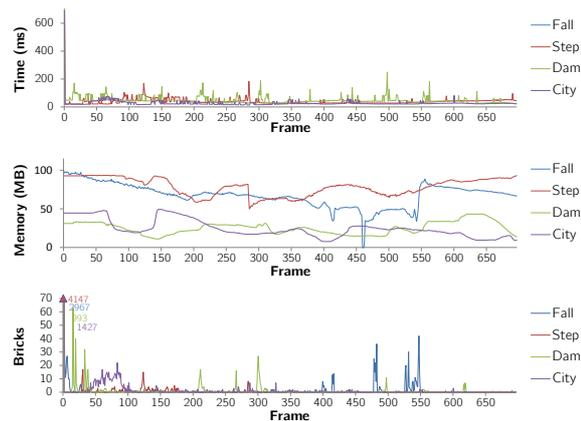
Figure 13: System behavior during data exploration of a single time step with different views and zooms. Note that the graph for uploaded bricks in the left column is capped at 50 for better visualization, with the number of bricks in the first frame explicitly labeled.
