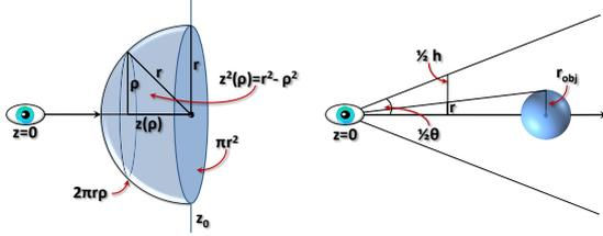
Figure 5: Quantities used in the estimation of the local filter weights  $\lambda_{ij}$ . Left: Estimating  $\text{Var}[z]$ . Right: Estimating the screen space radius  $r$  from  $r_{obj}$ .
