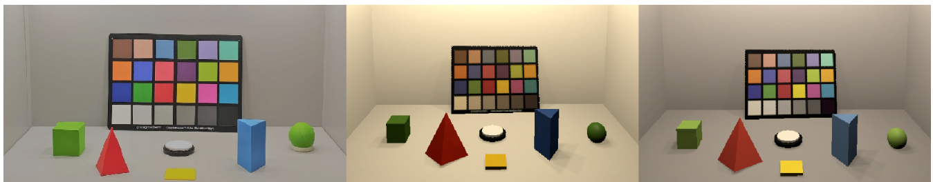
Figure 1: The quantitative experimental environment. Left: Scenario on a real light booth and real several objects created with a 3D printer; Center: Virtual environment with 3D scanned objects and RGB textures under D50 illuminant; Right: Virtual environment with 3D scanned objects and hyperspectral textures under D50 illuminant.
