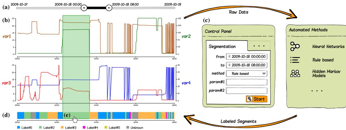
**Figure 1:** The Visual Analytics approach to time series segmentation: both raw data (b) and results (d) are depicted for a certain time interval (a). Several interactions allow inspecting the results (e). The user can steer automated segmentation (c) for selected time interval. [Single elements used from Basiliq UI images kit by Cloud Castle, licensed under Creative Commons.]
