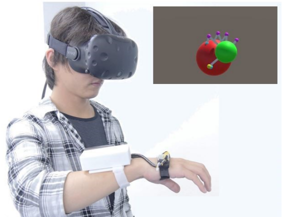
Figure 14: VR application with our prototyped device. The user grasps a boll in a virtual environment with their finger motion.
