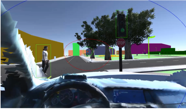
Figure 5: Our simulated automotive use case: the visibility of relevant objects (pedestrian, traffic light) in the peripheral view of the driver serve as input for assistive system functions (attention shift).
