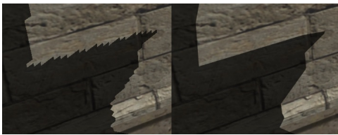
Figure 6: The image shows difference in quality between shadow mapping and shadow volumes.
