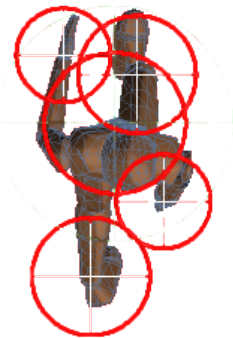
Figure 5: Collision model of 5 cylinders around the head, the left and right hands, and the left and right foot.
