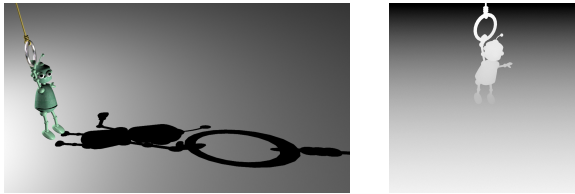
Figure 11: Shadow map for a point light source. Left: view from the camera. Right: depth buffer computed from the light source.
