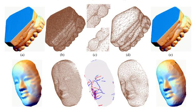
**Figure 12:** Top row: (a) the Teeth Casting model; (b) its wireframe image; (c) a magnified view of a part of the mesh before (top) and after (bottom) decimation; (d) a wireframe image of the model after decimation; (e) the decimated model. Bottom row: (a) a Noh mask model; (b) its wireframe image; (c) ridges and ravines detected on the model; (d) a wireframe image of the Noh mask model after decimation; (e) the decimated model. The models are flat-shaded to enhance the faceting effect.
