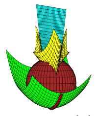
**Figure 1:** The elliptic paraboloid  $z = 3x^2 + y^2$  (green), its ridge (black), the caustic sheet (yellow) and the sphere of curvature (brown) associated with the maximal principal curvature at a ridge point, the skeleton (white).
