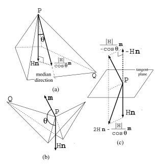
Figure 8: (a) The median and normal vectors lie on the same side from the tangent plane: moving in the median direction with normal speed component equal to the mean curvature. (b) The median and normal vectors lie on the opposite sides from the tangent plane may happen for saddle vertices. (c) Computation of the speed vector in (b).
