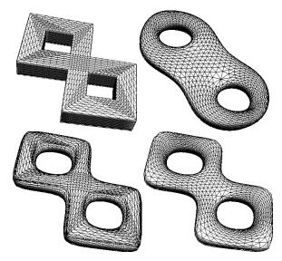
**Figure 9:** Top-left: a polygonal two-holed torus consisting of parts with different sampling rates. Top-right: Laplacian smoothing improves the mesh sampling rate but substantially deforms the initial shape. Bottom-left: the mean curvature flow <sup>6</sup> increases mesh irregularity. Bottom-right: smoothing according to (6) produces a regular meshing surface whose shape is close to the shape produced by the mean curvature flow.
