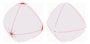
Figure 3: Positive maxima of the maximal principal curvature along its normal section curve (left) and curvature line (right) on a polygonal model of a rounded octahedron oriented by its inward normal.
