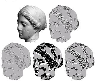
Figure 6: Top-left: the Venus model (courtesy Cyberware). Top-right: ridges and ravines are marked by the black and white strokes, respectively. Bottom: ridge and ravine triangles detected on the Venus model (left), after adding several layers of surrounding triangles (middle), after thinning (right).
