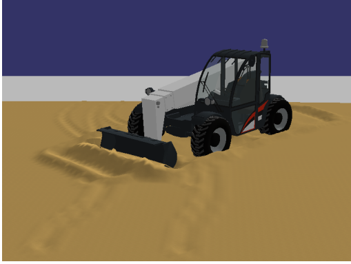
Figure 2: A telescopic manipulator, acting as a bulldozer, pushes sand horizontally. Wheel trails, can also be observed.
