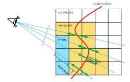
**Figure 1:** Macro-voxel marking: Initially all cells are set to notempty and not-intersected. Threads are assigned to rays and execute multi-level DDA on the higher level macro-voxel grid. Before finding a macro-voxel overlapped by the truncation interval, macro-voxels are marked as empty. When the truncation interval overlaps with the cell, the macro-voxel is marked as intersected.
