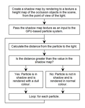
Figure 2: Flowchart detailing our approach.
