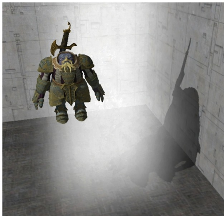
A shadow mapped object, casting a shadow onto the background with no shadow cast onto the smoke particle system.
