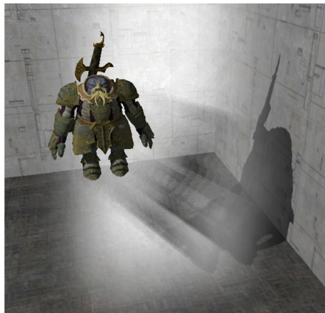
The addition of shadows that are cast onto the smoke (2D semi-translucent billboards) and interact with it adds realism to the scene. The current prototype – based on the DirectX SDK sample framework – still suffers from typical shadow mapping artifacts .
