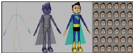
Figure 5. From the left: bone structure, polygon mesh, skin with textures and facial morph targets
