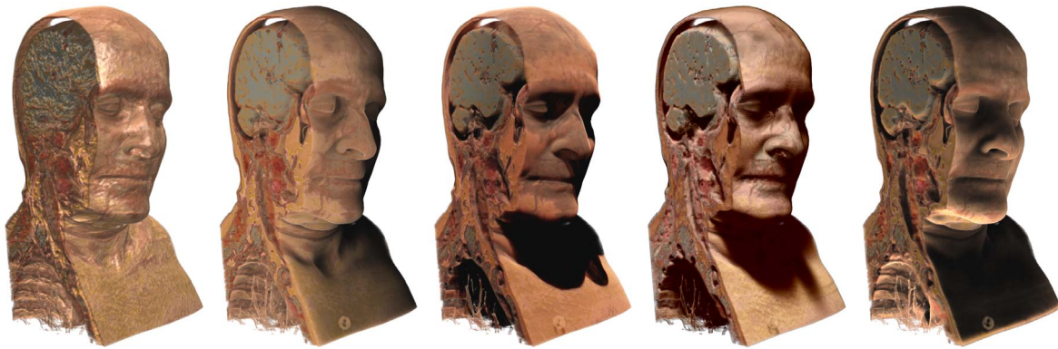
Figure 3: Visual comparison when applying different volumetric illumination models. From left to right: gradient-based shading [Lev88], directional occlusion shading [SPH*09], image plane sweep volume illumination [SYR11], shadow volume propagation [RDRS10b] and spherical harmonic lighting [KJL*12]. Apart from the used illumination model, all other rendering parameters are constant.
