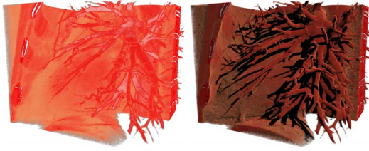
Figure 1: Comparison of a volume rendered image using the local emission absorption model [Max95] (left), and the global half angle slicing technique [KPHE02] (right). Apart from the illumination model, all other image parameters are the same.
