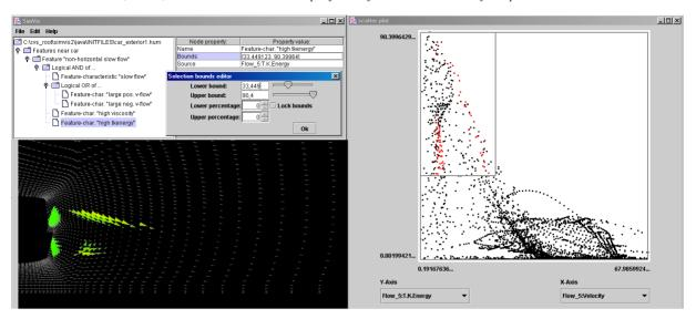
**Figure 8:** Step 3 of analysis: another AND refinement, further restricting to high values of turb. kinetic energy, performed in the tree viewer. Only parts with strong rotational component are in focus. (see also colorplate)
