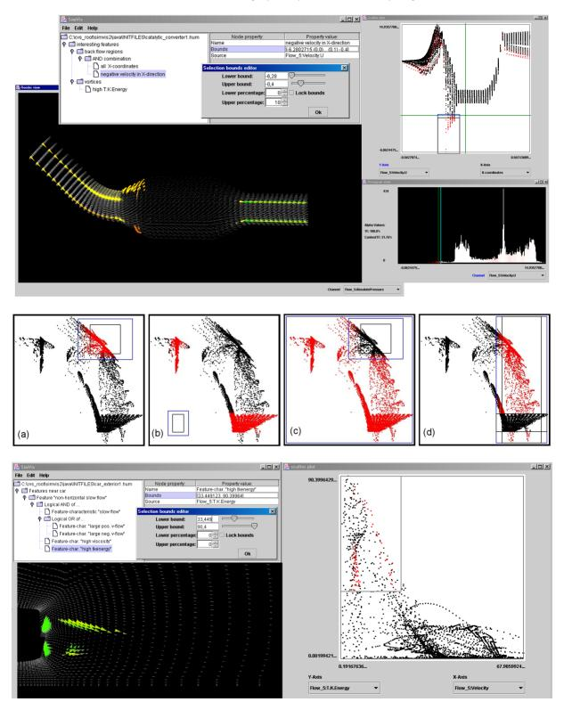
**Figure 10:** Two examples for feature-based flow visualization using our framework for interactive feature specification and four illustrations of different combination modes for smooth brushes (middle row) (for verbose captions see figures 1, 3, and 8).
