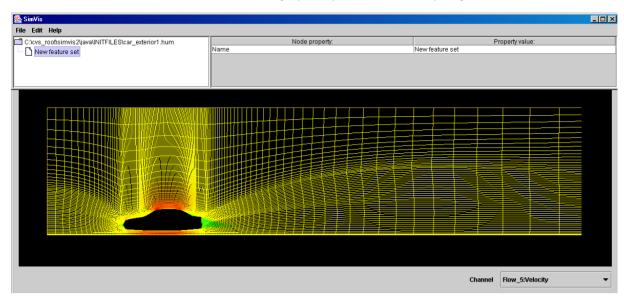
**Figure 5:** Air-Flow around a moving car: After loading the data set, an empty feature set is created, and the spatial layout of the data is shown, overall velocity information is mapped to color (green denotes low, red high velocity).
