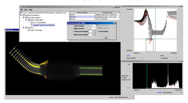
**Figure 1:** Flexible Feature Specification: simulation data of a catalytic converter is shown, two features have been specified based on our feature definition language, using the different views for interaction and visualization. (see also colorplate)
