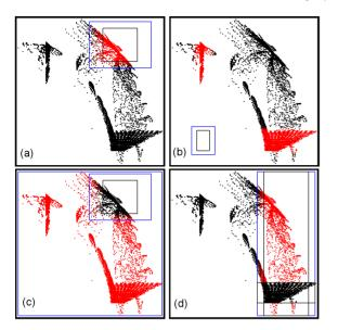
**Figure 3:** four examples of 2D brush types which users found useful during interactive analysis (catalytic converter example, pressure [x] vs. velocity [y]): (a) "high velocity and high pressure" (logical AND), (b) "low velocity or low pressure" (log. OR), (c) "all but high vel. and high pressure" (NOT-AND), and (d) "high pressure but not low velocity" (SUB = AND-NOT). (see colorplate for shades of red)
